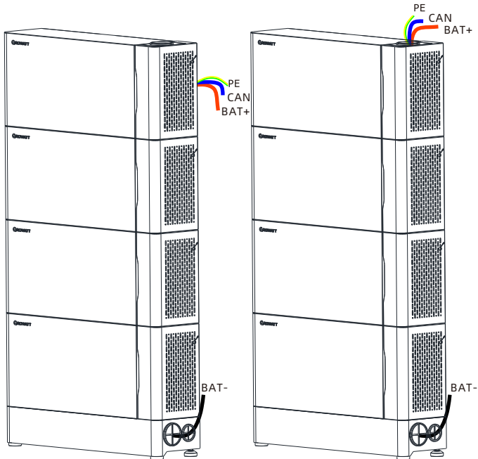
Figure 4.18: Trim cover installation is completed
